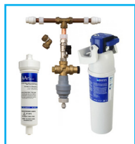
Installation Rail for hard water areas. This includes a carbon block candle for the chilled water inlet & a scale removal filter for the hot water inlet
