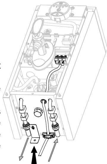
Vent & overflow      4th fixing      Cold water inlet
