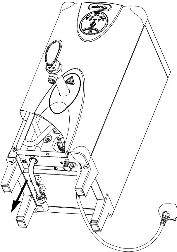
If the boiler is required to drip or overflow into the drip tray, the configuration of pipework may be altered as follows. Remove the machine front panel and unclip the pipework elbow. Carefully pull the elbow in the direction of the arrow, out of the silicone connecting tube on the end of the main water pipe. The silicone connecting tube will now direct water into the drip tray.
