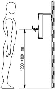
To comply with recommendations from the Health and Safety Executive it is important that due consideration be given to safe operation of the controls of the boiler. The boiler should therefore be mounted in such a manner that the operator can stand directly facing the machine with the controls at a recommended height from the floor to the draw-off tap handle of 1200mm +/- 100mm. Consideration should also be
